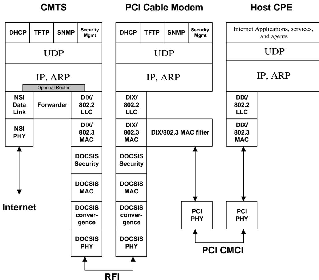
Figure 3–5 - End-to-End PCI Cable Modem Protocol Stack
