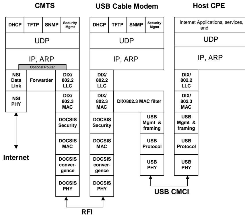
**Figure 3–3 - End-to-End USB Cable Modem Protocol Stack**
