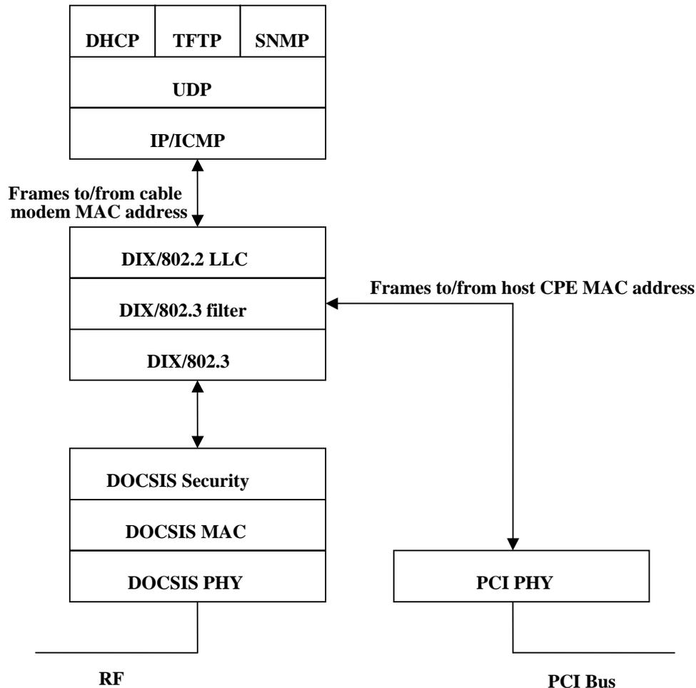
**Figure 3–4 - Protocol Stack for Internal Cable Modems**
