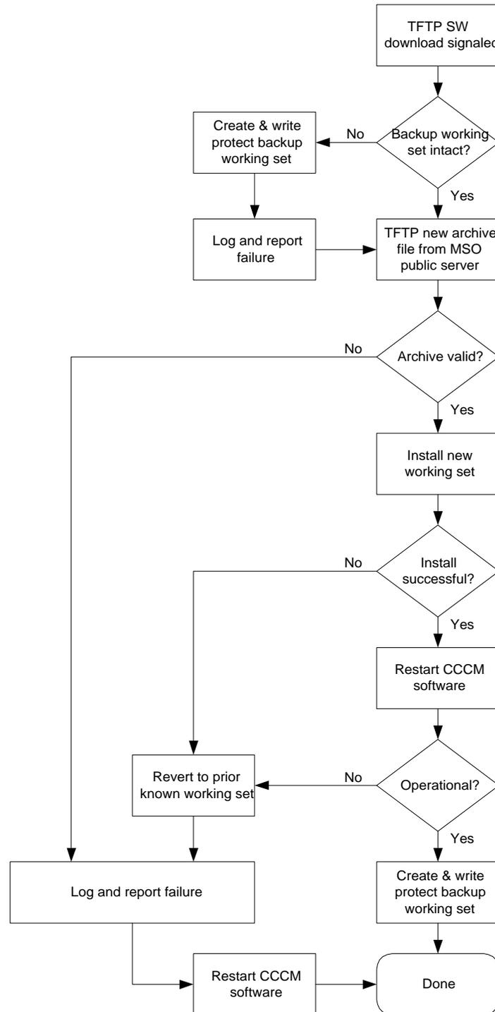
**Figure C-2 - Downloading Cable Modem Operating Software**
