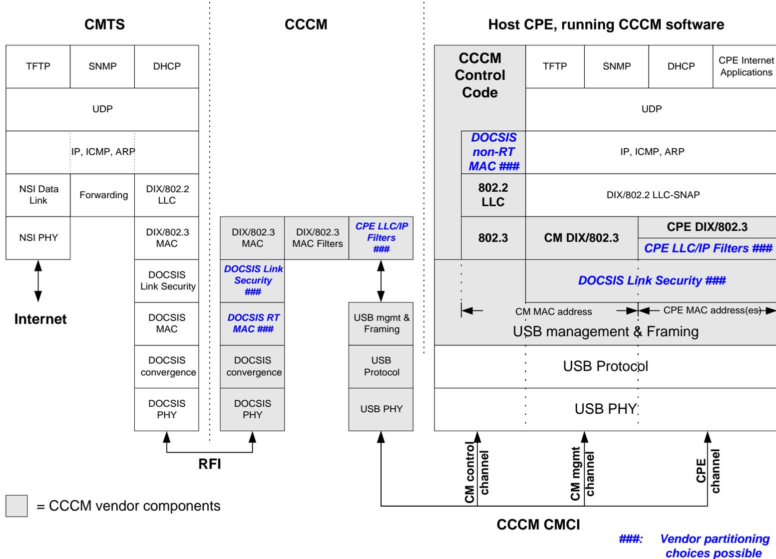
Figure 4-4 - End-to-End USB CCCM Protocol Stack
