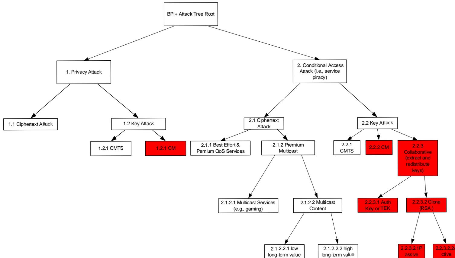
Figure E-1 - BPI+ Attack Tree (attacks whose effectiveness is impacted by the introduction of CPE-controlled CMs are highlighted in red).
