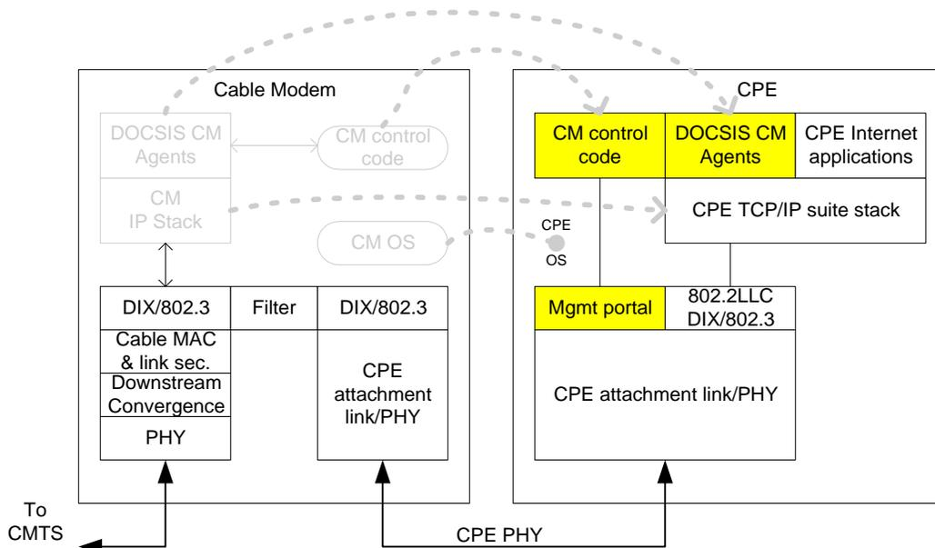
**Figure C-1 - CPE Controlled Cable Modem (CCCM) functional migration**
