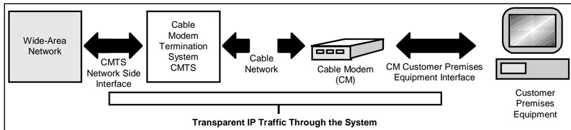
**Figure 1–1 - Transparent IP Traffic through the Data-Over-Cable System**
