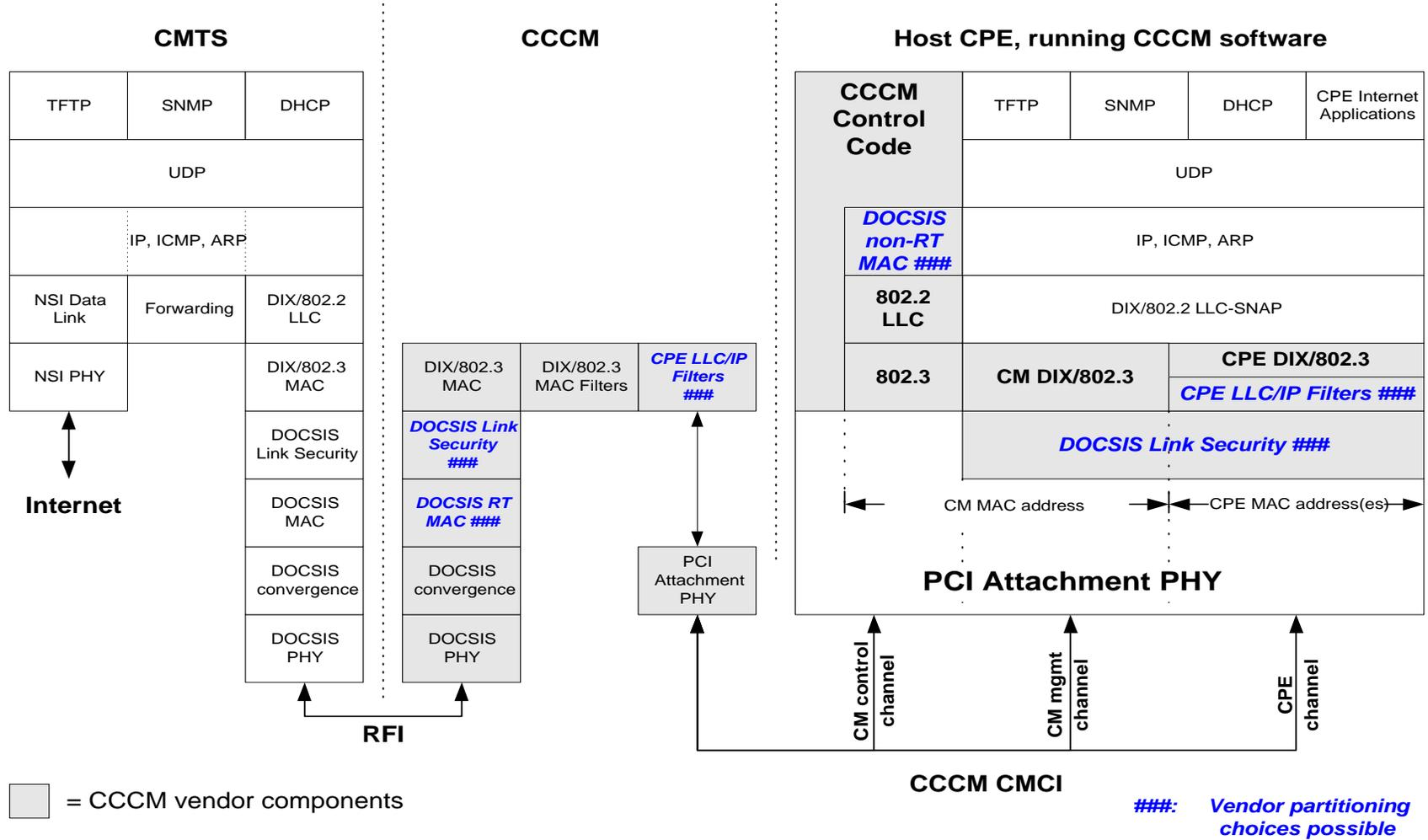
Figure 4-3 - End-to-End PCI CCCM Protocol Stack
