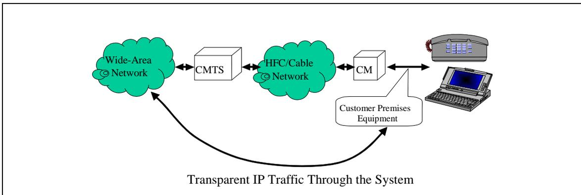
**Figure 1. Transparent IP Traffic Through the Data-Over-Cable System**
