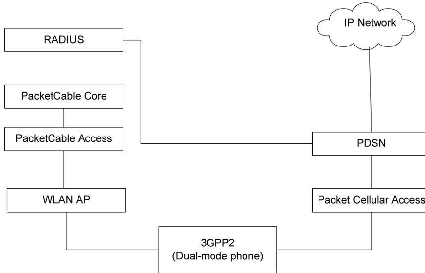
**Figure 4 - PacketCable Interfaces to 3GPP2 Packet Cellular Networks**
