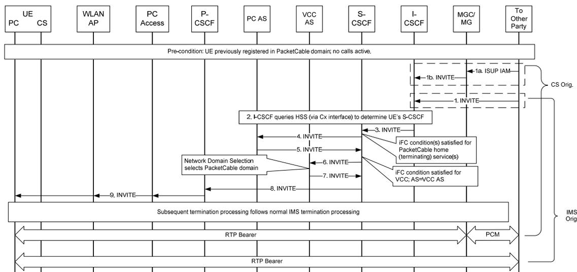
**Figure 17 - UE Termination Call Setup in PacketCable Domain**
