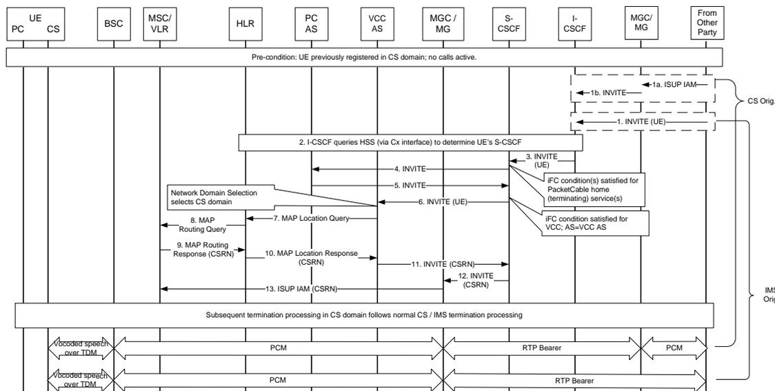
**Figure 18 - UE Termination Call Setup in CS Domain**
