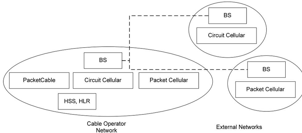
**Figure 5 - Scenario 1: PacketCable operator owns a CS/PS network**
