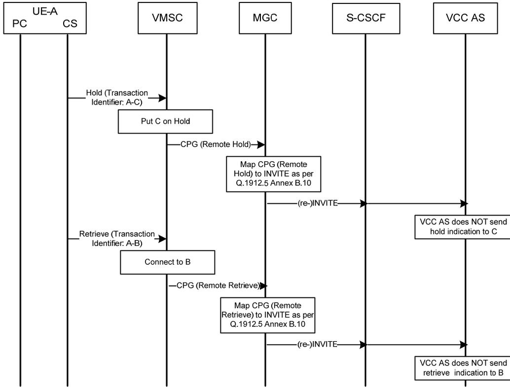
**Figure 27 - PacketCable to 3GPP CS Transfer of Call Hold, A-B active prior to transfer, A-C was VCC AS initiated (2 of 2)**
