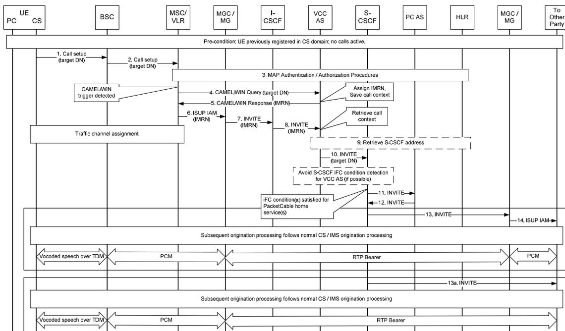
**Figure 16 - UE Origination Call Setup in CS Domain**
