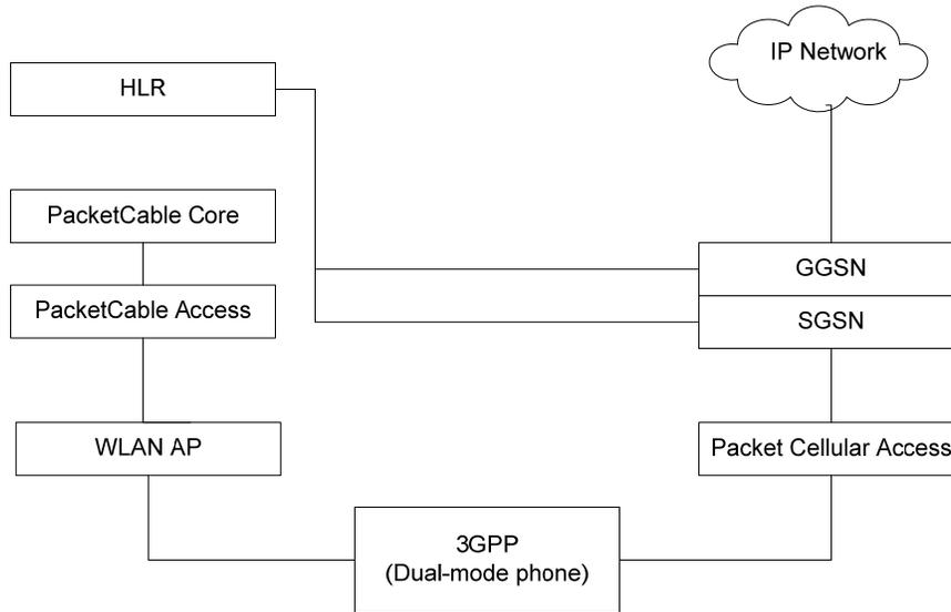
**Figure 3 - PacketCable Interfaces to 3GPP Packet Cellular Networks**
