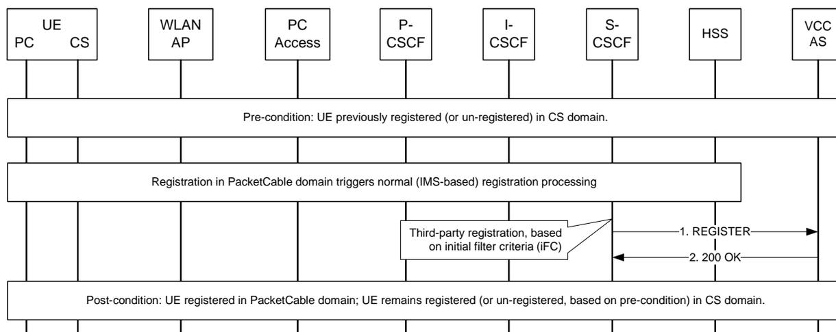
**Figure 12 - UE Registration in PacketCable Domain**
