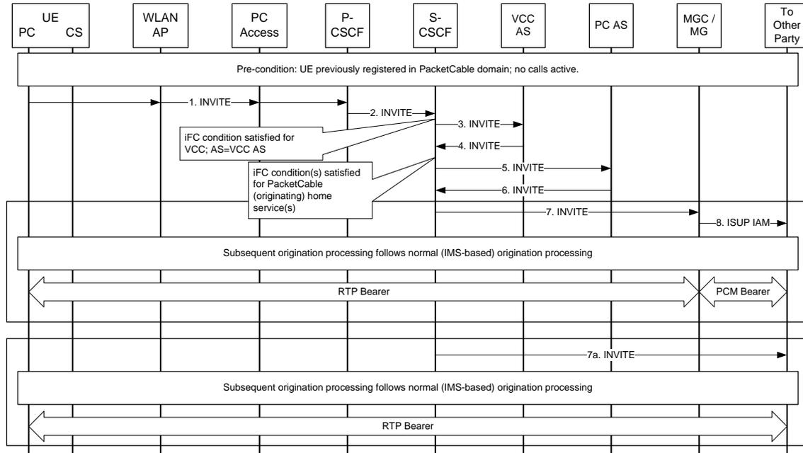
**Figure 15 - UE Origination Call Setup in PacketCable Domain**
