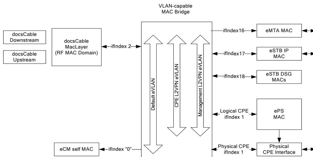
**Figure III–1 - L2VPN Embedded VLAN (eVLAN) Model**
