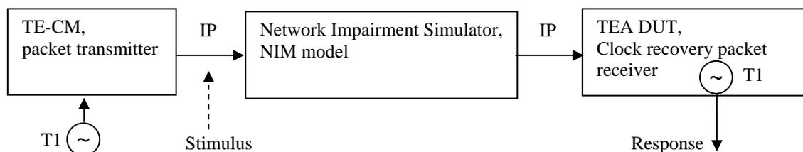
**Figure 6–5 - Clock Recovery - Performance Test Environment**
