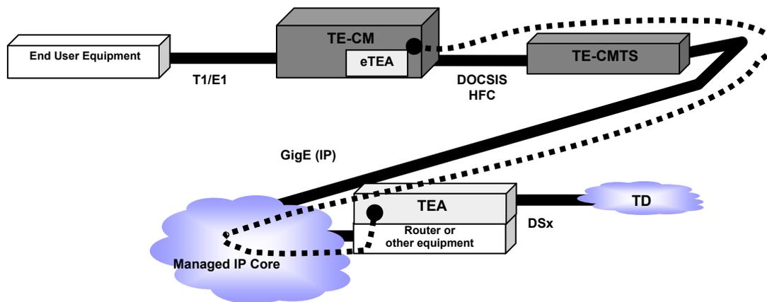
Figure 5-6 - T1 to TDM core, IXC or PSTN
