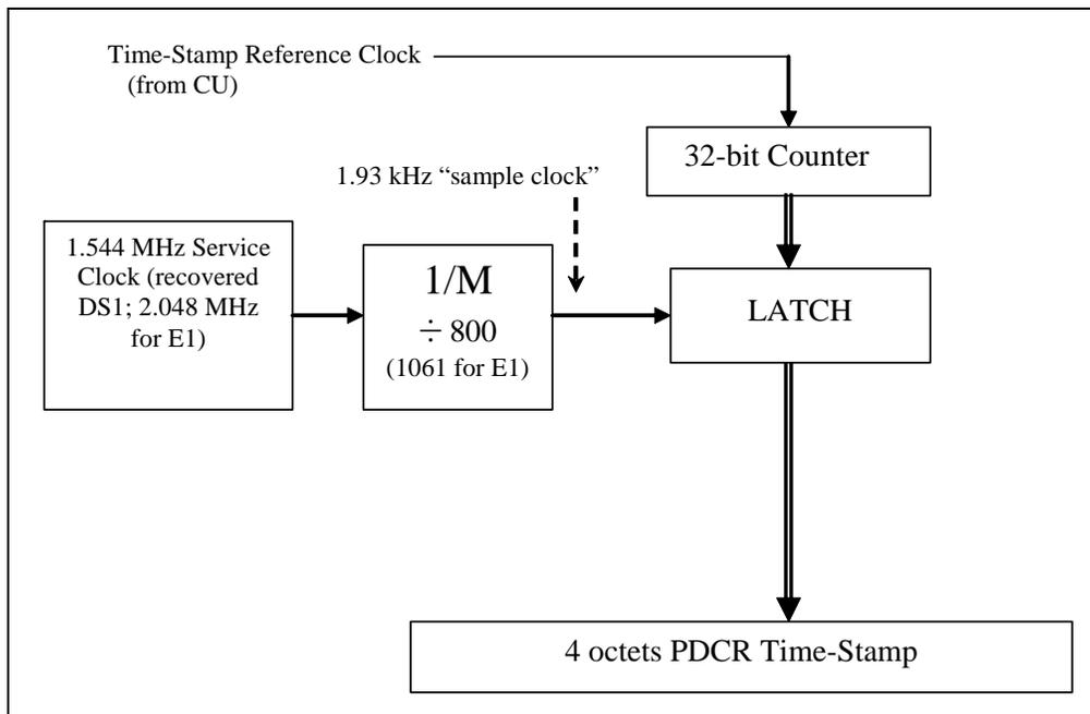
**Figure 6-4 - Description of PDCR "transmit" function**
