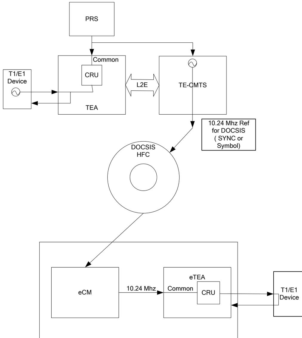
**Figure V-2 - Prime Differential Clock Recovery**
