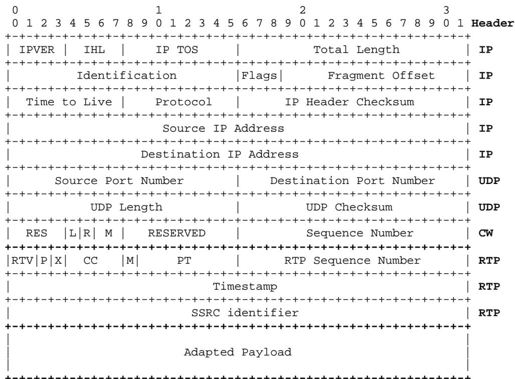
**Figure 6–1 - Header Format (Only IPv4 shown)**
