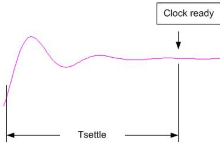
**Figure 6-7 - Clock recovery settling time**
